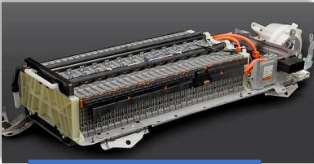
Toyota Prius Hybrid - NiMH Battery
